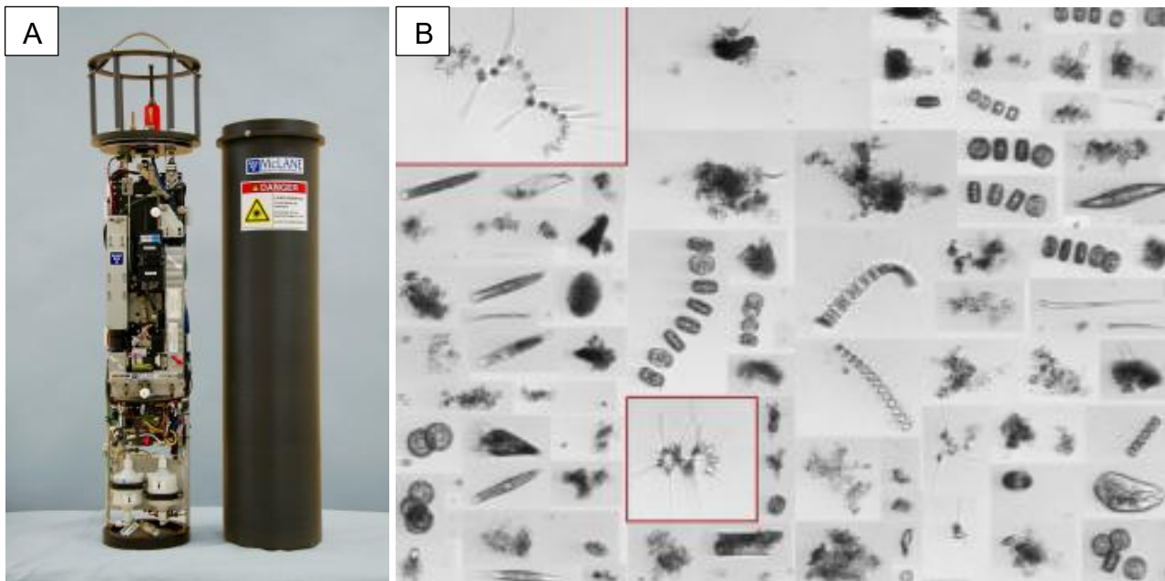
Figure 26. The Imaging Flow Cytobot (A) and (B) a mosaic of phytoplankton and microzooplankton images from the July 2025 IFCB deployment in the CMS.
