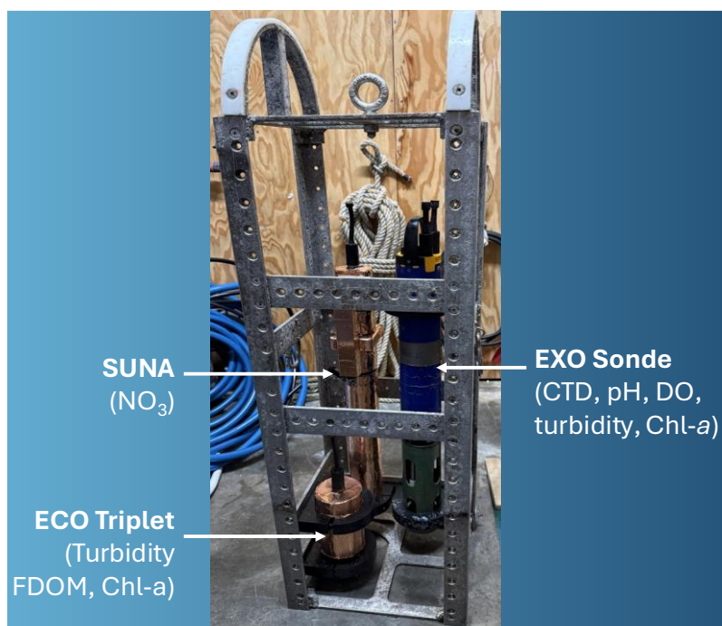
Figure 6. The instrument frame as deployed in Dec 2025.
